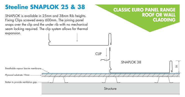
38mm high wall cladding can be installed on battens at 600mm centres with no substrate required.
